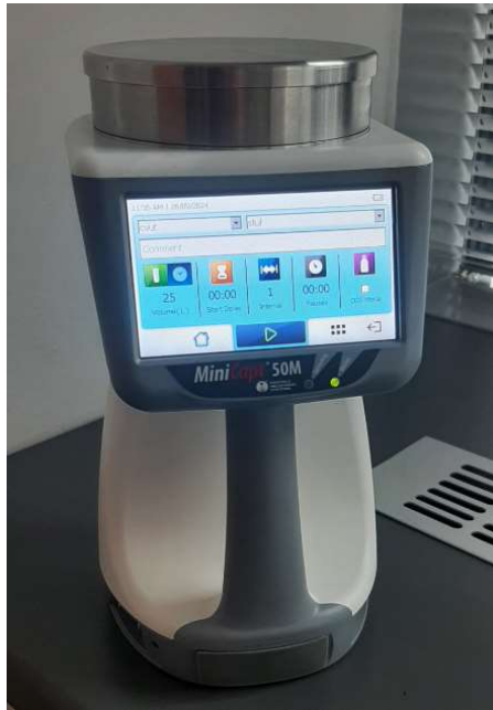
Figure 5 - Aeroscope for active air monitoring
