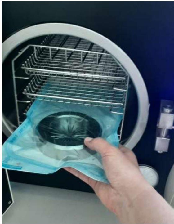
Figure 13 - Impactor placed in a sterilization bag for sterilization in an autoclave
