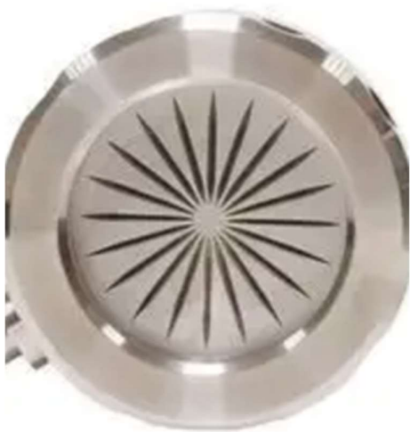
Figure 2 – The impactor of the aeroscope and its "star"
